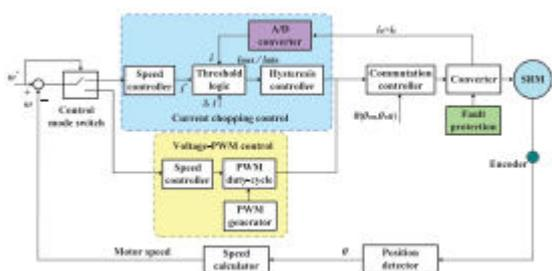
Fig. 6. SRM control strategy under single-source driving mode.
