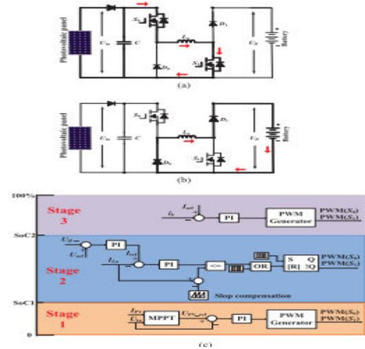
Fig. 10. Mode 6 charging states and control strategy. (a) Phase inductance charging. (b) Battery charging. (c) Charging control strategy.
