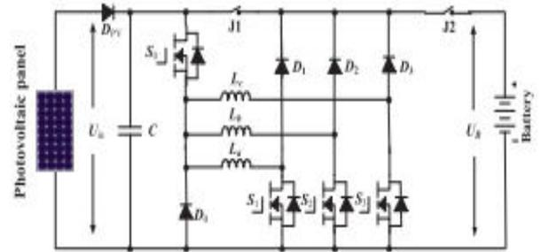
Fig. 2. Proposed tri-port topology for PV-powered SRM drive.
