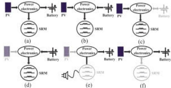
Fig. 3. Six operation modes of the proposed tri-port topology. (a) Mode 1. (b) Mode 2. (c) Mode 3. (d) Mode 4. (e) Mode 5. (f) Mode 6
