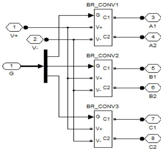
Fig 12 Three phase converter
