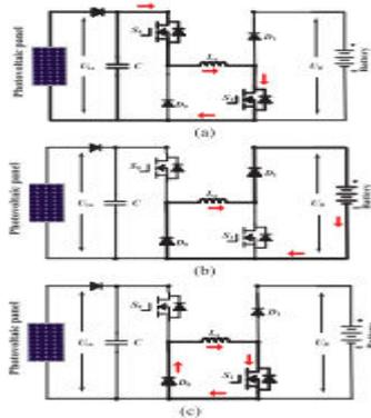
Fig. 7. Mode 1 working states. (a) Winding exciting state. (b) Battery charging state. (c) Freewheeling state
