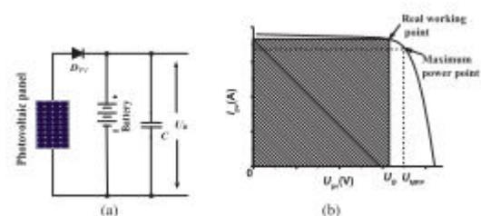
Fig. 4. Power supply at mode 2. (a) Compound power source. (b) Working point of the PV
