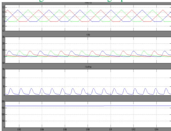
Fig 14 Simulation results of single-source driving mode Flux, Current, Torque, Speed
