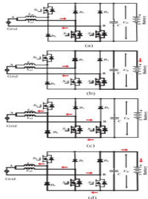
Fig. 9. Mode 5 charging states. (a) Grid charging state 1 ( $U_{grid} > 0$ ). (b) Grid charging state 2 ( $U_{grid} > 0$ ). (c) Grid charging state 3 ( $U_{grid} < 0$ ). (d) Grid charging state 4 ( $U_{grid} < 0$ ).
