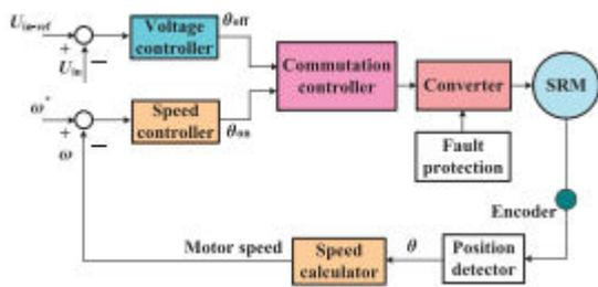
Fig. 8. Control strategy under driving-charging mode (mode 1).
