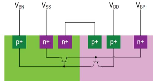
Figure 3: Leakage path in forward body biasing
