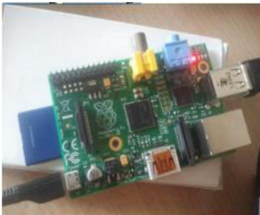
Fig.2 Raspberry pi processor
