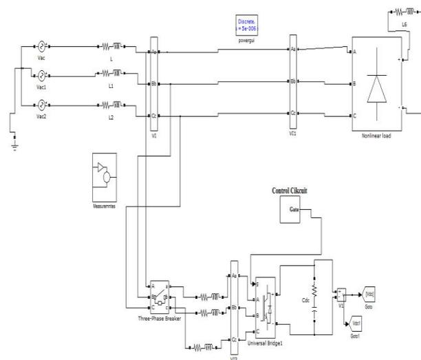
Fig.6. Matlab/Simulink circuit for Power system with D-STATCOM
