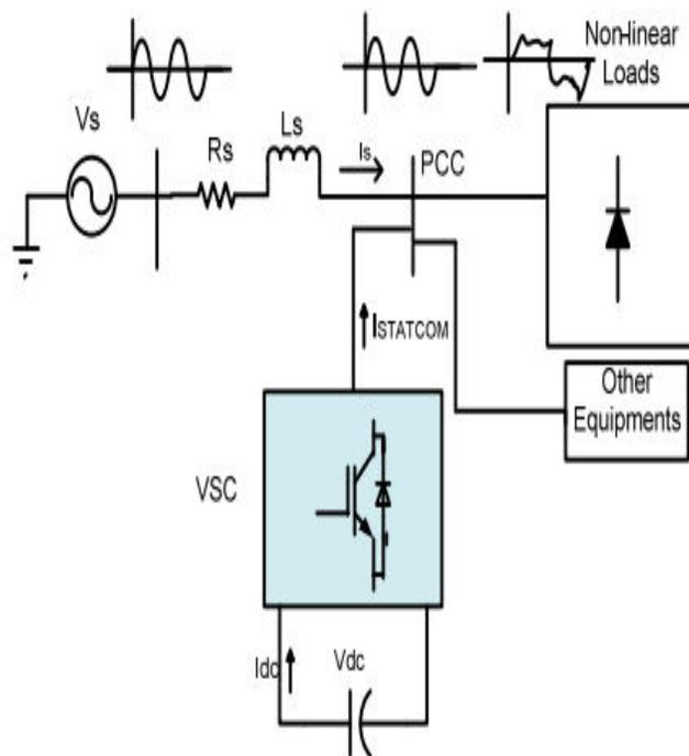
Figure.3: Power system with D-STATCOM
