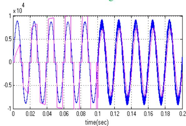
Fig. 13. Power factor angle between source voltage and current
