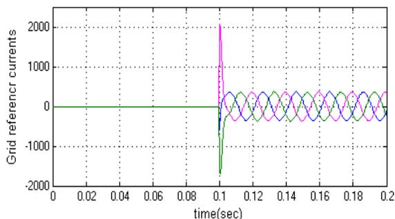
Fig. 7. Simulation waveform for Grid reference current
