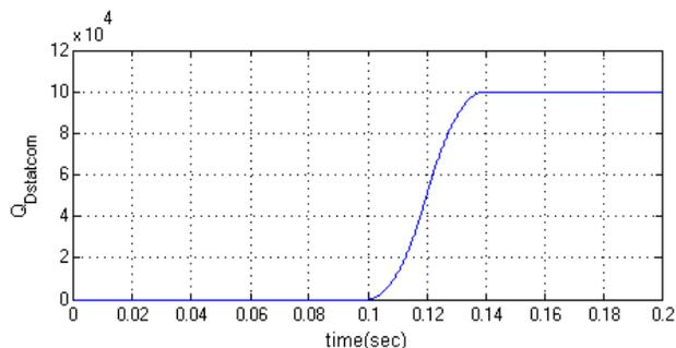
Fig. 11. Reactive power supplied by D-STATCOM
