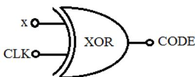
Fig. 3 Encoded Data With Xor
