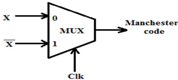
Fig. 6 Manchester Encoder With Balance Logic
