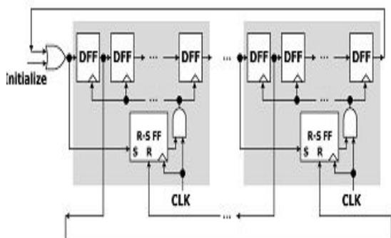
The above block diagram shows the power controlled Ring counter. First, total block is divided into two blocks. Each block is having one SR FLIPFLOP controller
