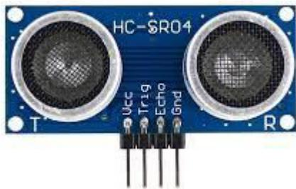
**Fig 2: Ultrasonic sensor**
