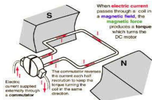
Fig 5: DC motor working principle
