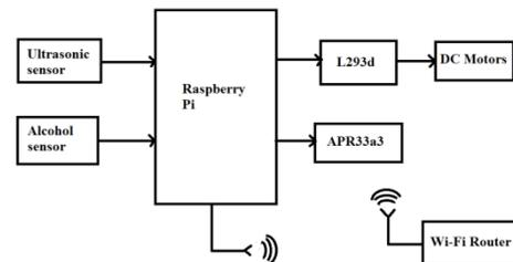
**Fig 1: Block diagram of Design and implementation of accident preventing, driver intoxication finding system using feedback and IoT**
