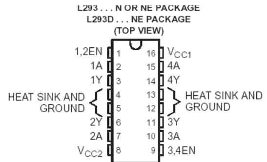
Fig 4: L293d driver IC
