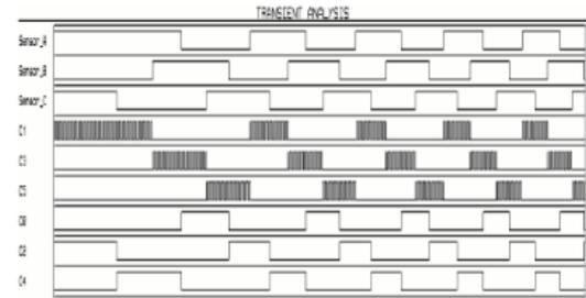
**Fig. 6 Pulses to drive the MOSFETs** The pulses shown in the figure are fed to the 24V, 80 W, 1500 rpm BLDC motor and the motor voltage equivalent to 1500 rpm speed is shown in figure.
