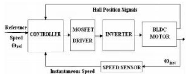
Fig 2. Schematic diagram of BLDC motor drive
