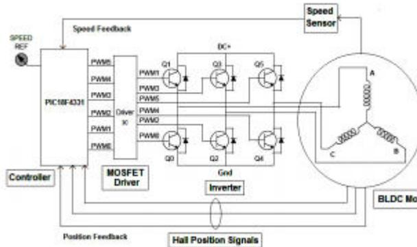
Figure 3. PIC184331 microcontroller based BLDC motor drive
