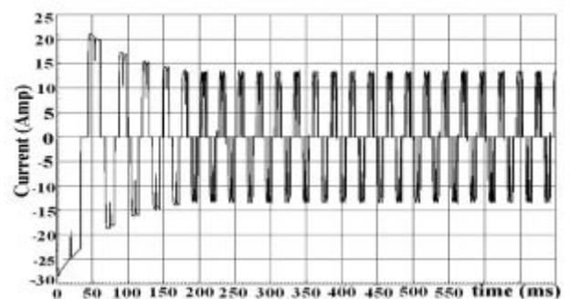
**Fig 8. Simulation result for phase current response of BLDC motor on full load (1151 rpm)**
