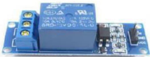
Figure 3: Relay module
