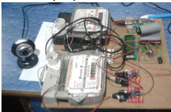
The Raspberry Pi 3 provides a supply of 5 V but the electrical appliances in general operates on 230 V. So relays are employed in this system for voltage conversions and also to remotely ON and OFF the electrical appliance. The energy consumed by the two
