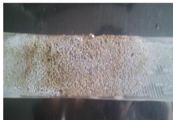
Fig 2 Aluminum 6061 and acrylic sheet bonding (flexi kwik)
