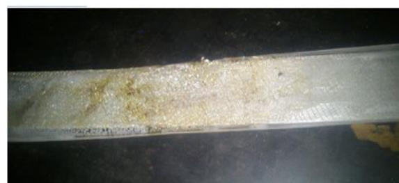
Fig 3 Aluminum 6061 and acrylic sheet bonding (flexi kwik)
