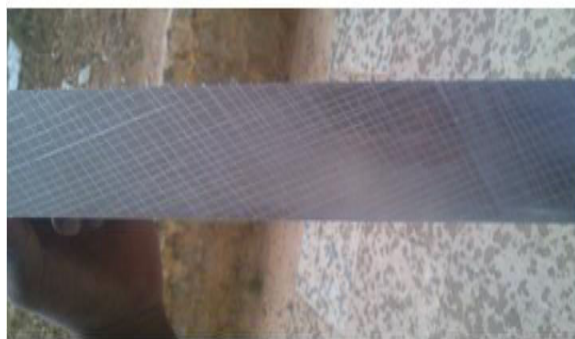
Fig1. Aluminum 6061 diamond knurling
