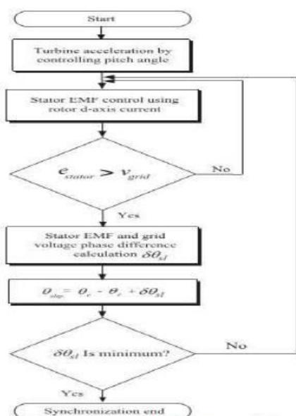
Fig. 5. Sequence of DFIG synchronization
