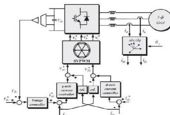
Fig. 6. Control block diagram of grid-side converter.
