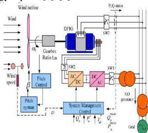
Fig. 1 Basic configuration of DFIG wind turbine system
