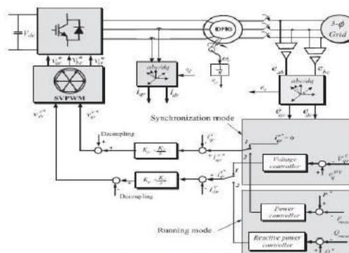
Fig. 2.Active and reactive power control for synchronization mode and running mode.
