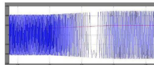
Fig.10 Rotor current variation due to speed transition
