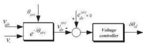
Fig. 4. Phase difference compensation for synchronization
