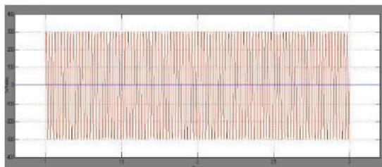
Fig.14 Grid Voltage under L-G Fault with Series Compensator
