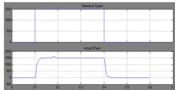
**Fig: 9. Reference speed and actual speed in rpm.**
