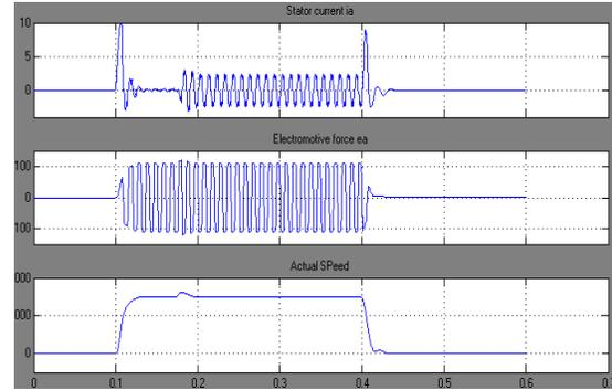
**fig 8 Output model of the Simulink: stator current, back emf, actual speed.**
