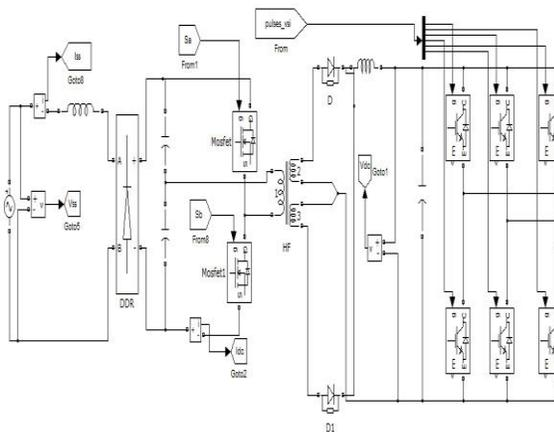
**Fig 2.Simulation circuit of Proposed BLDC motor drive with front-end BL buck-boost converter**
