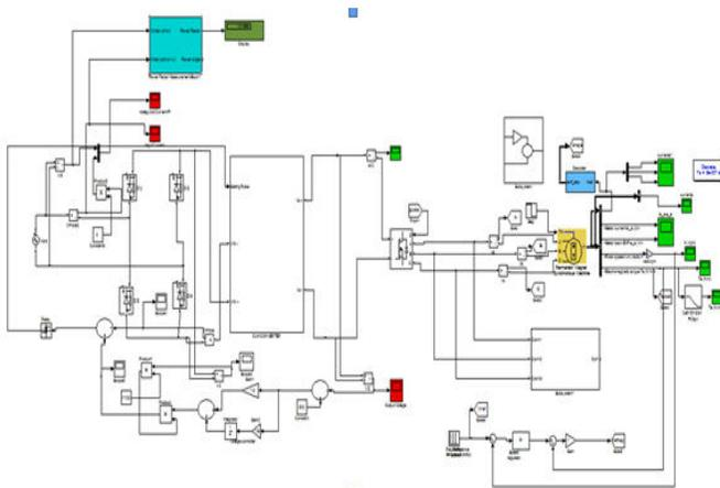
**Fig7.1: Simulink model of the PFC based BLDC drive.**
