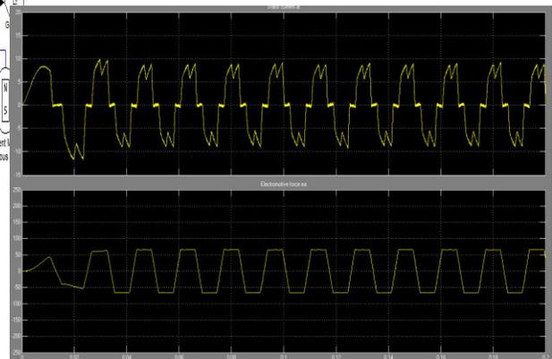
**Fig5. stator current and stator back emf of BLDC motor**
