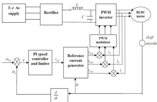
**Fig 2. PI speed controller of the BLDCM drive**
