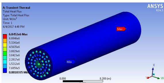
predict the temperature distribution in heat transfer analysis in both the shell and tube.
