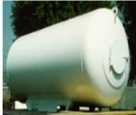
**Fig 1.1. Cylindrical Pressure Vessel**
