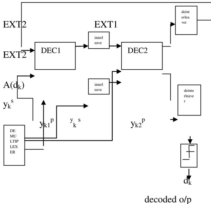
Figure 3 Turbo Decoder Structure.
