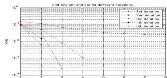
FIG 5 BER vs. SNR plot for turbo codes for different iterations
