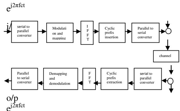
Fig 1 Block diagram of a basic OFDM transceiver.
