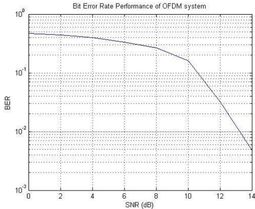
FIG 6 BER of OFDM vs SNR
