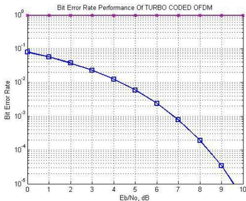
FIG 7 BER Performance Of Turbo Coded OFDM
