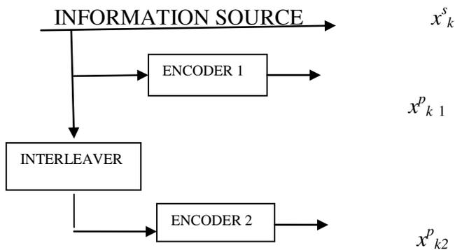
Figure 2 - Structure of a turbo Encoder
