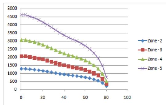
Fig:8 Base shear at different levels in various zones along X-Direction
