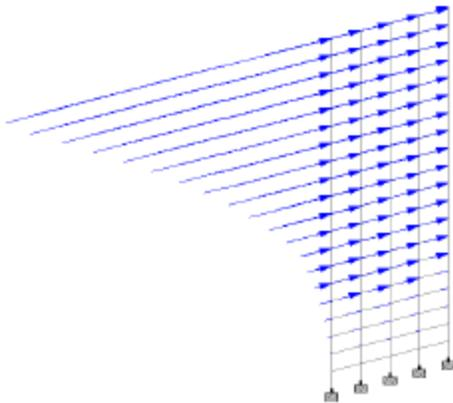
Fig: 7 Static loading in a single frame
