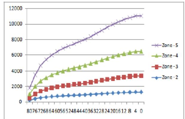
Fig: 9 Base shears at different levels in various zones along Z-Direction
