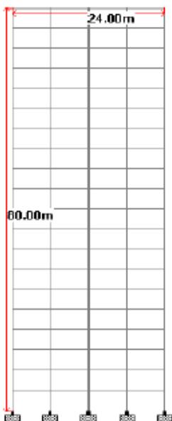
Fig: 1 20 storey Model Structure for analysis
