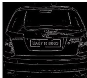
(c) Edge detection by sobel operator
