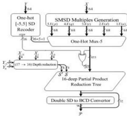
Fig 1: Block diagram of the proposed multiplier.
