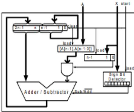
**Fig 3: Multiplier block diagram with SBR input**
