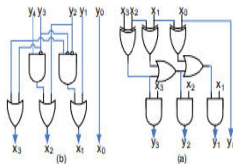
Fig 2: a) 2'sc to SBR encoder (4 bit)
