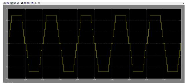
Fig. 4 Output waveform of nine level cascade H bridge multilevel inverter
