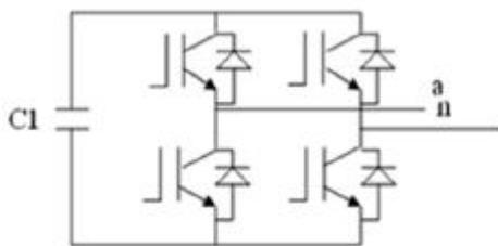
Fig. 1 Cascade H bridge multilevel inverter
