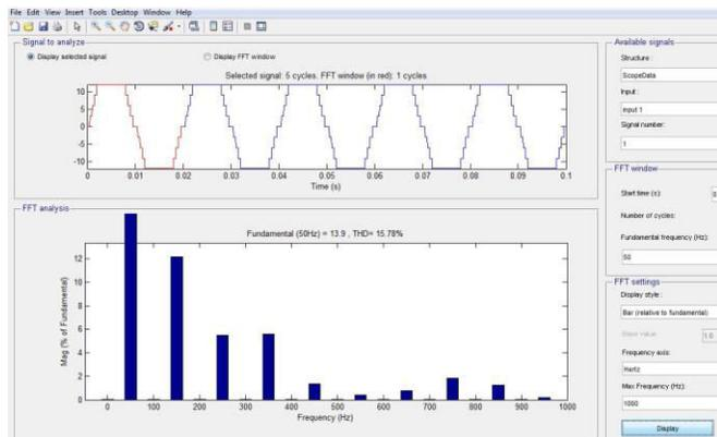
**Fig. 5** FFT analysis of nine level inverter
