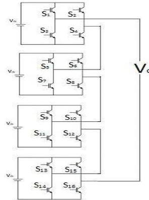
Fig. 2 Conventional diagram of nine level cascade H bridge multilevel inverter
