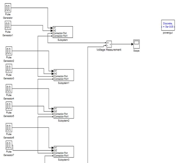
Fig. 3 Simulation diagram of nine level cascade H bridge multilevel inverter
