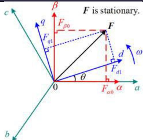
Fig. Coordinate transformation of dc components
