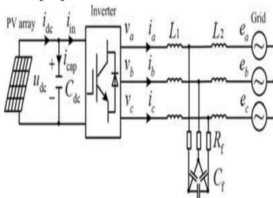
Fig. 1 Transformerless three-phase PV inverter system
