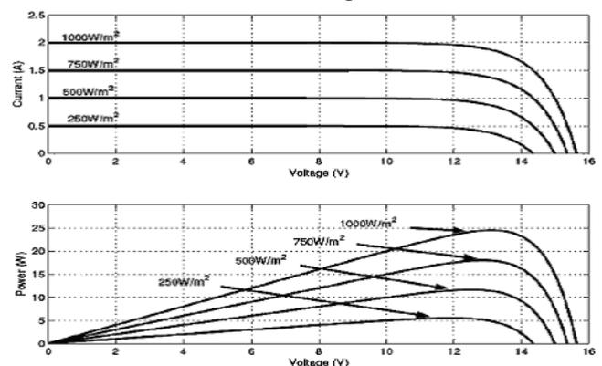
Fig : The I-V and P-V characteristics of a solar cell including the effects of irradiance
