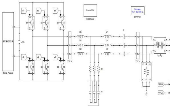
Fig. Transformerless three-phase PV inverter system Simulation
