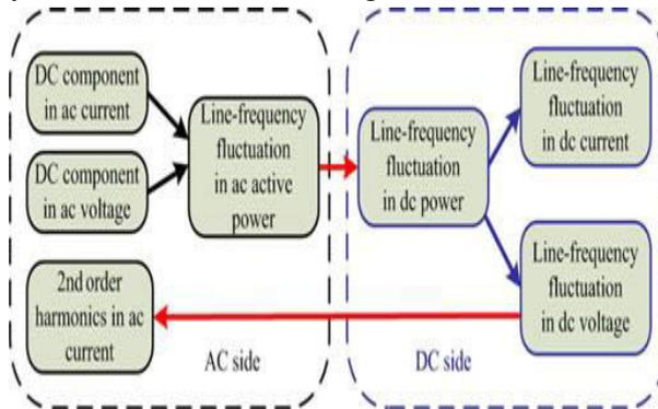
Fig. Influences of dc component on PV systems
