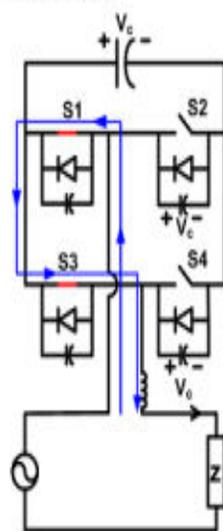
Fig 7. Mode III of ZVS operation
