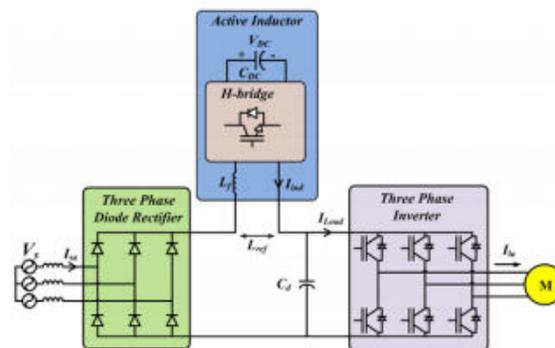
**Fig 2: Proposed ASD with an Active Inductor as DC-link reactor**
