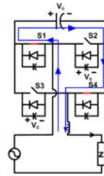
Fig 9. Mode V of ZVS operation
