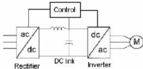
**Fig 1. Schematic diagram of Adjustable Speed Drive**
