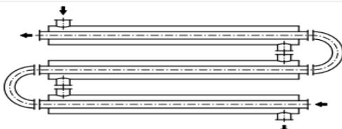
Figure 1 :Countercurrent double-pipe heat exchanger
