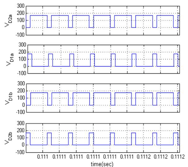
Fig.11 Experimental waveforms. (a)  $V_d$ s,  $I_{in}$ ,  $V_{out}$ ,  $V_{in}$ . (b) Diodes voltage:  $V_{d2a}$ ,  $V_{d1a}$ ,  $V_{d1b}$ ,  $V_{d2b}$ .
