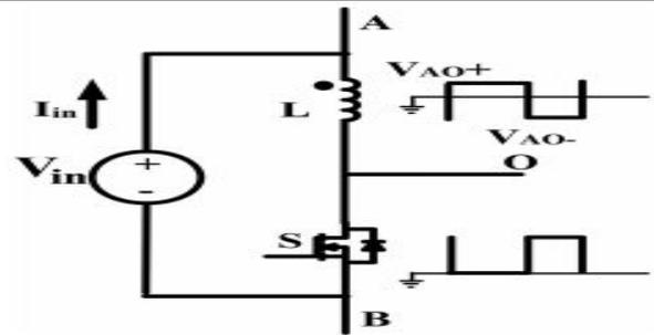
Fig.3. Inductive three-terminal switching core
