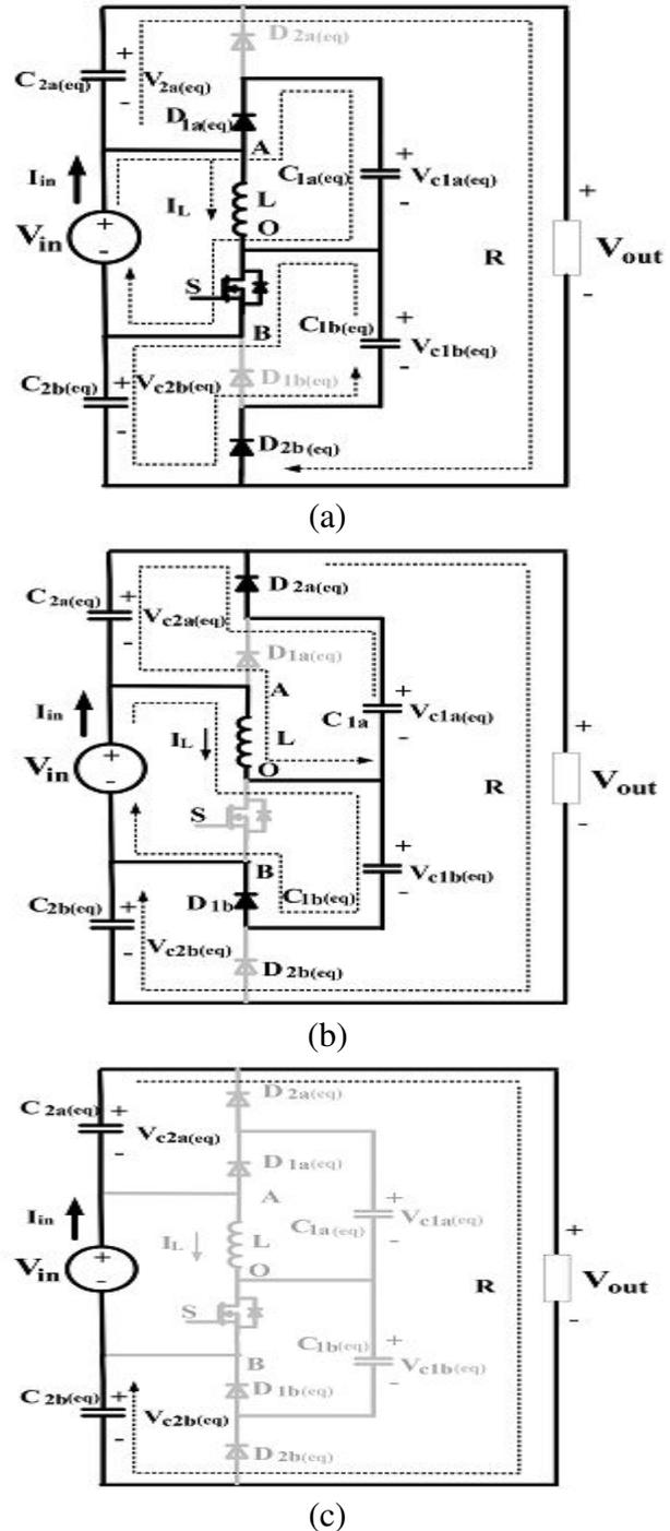
Fig.6. Three operation states. (a) State 1[0, DTs]. (b) State 2[DTs, (D+D1)Ts]. (c) State 3[(D+D1) Ts, Ts]
