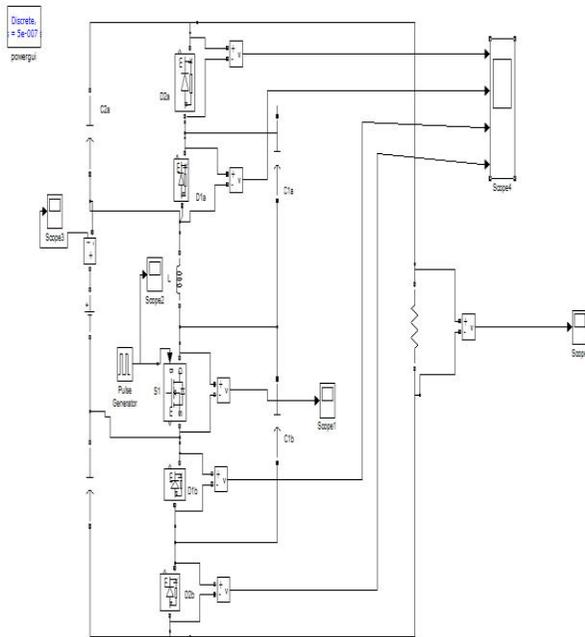
Fig.10 MATLAB/SIMULINK circuit for hybrid boost converttr
