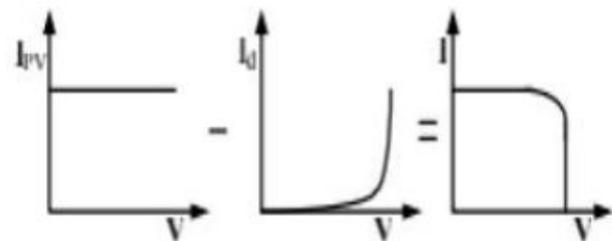
Fig.9 Characteristics I-V curve of the PV cell.
