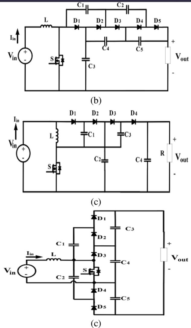
Fig.1. Previous high-gain dc–dc converters with single-switch single-inductor and proposed topology. (a) Boost + Dickson multiplier [16], (b) Boost + Cockcroft–Walton multiplier [16], (c) super lift with elementary circuit [18], (d) central source multilevel boost converter [21], (e) Cuk derived[22], (f) Zeta derived [22], (g) modified voltage lifter [23], and (h) proposed second-order HBC.
