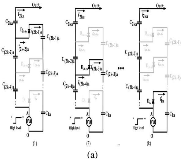
**Fig.4. Operation modes of even-order BVM positive branch. (a) State 1[0, DTs]. (b) State 2[DTs, Ts]**
