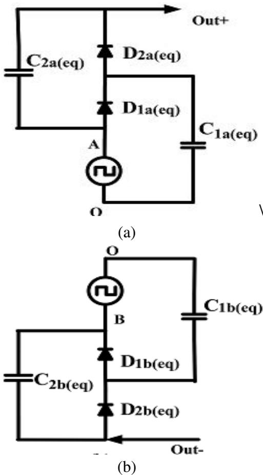
Fig.5. Equivalent circuit. (a) Even-order positive multiplier. (b) Even-order negative multiplier
