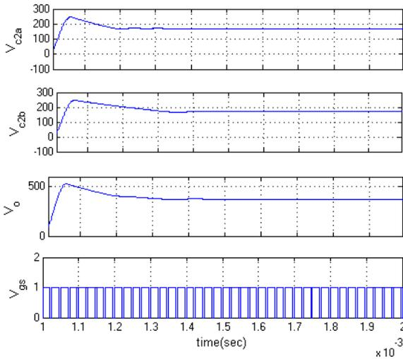
Fig.12. Experimental waveforms of voltage ripples:  $V_{c2a}$ ,  $V_{c2b}$ ,  $V_{out}$  and driving signal  $V_{gs}$  under (a)  $D=0.5$
