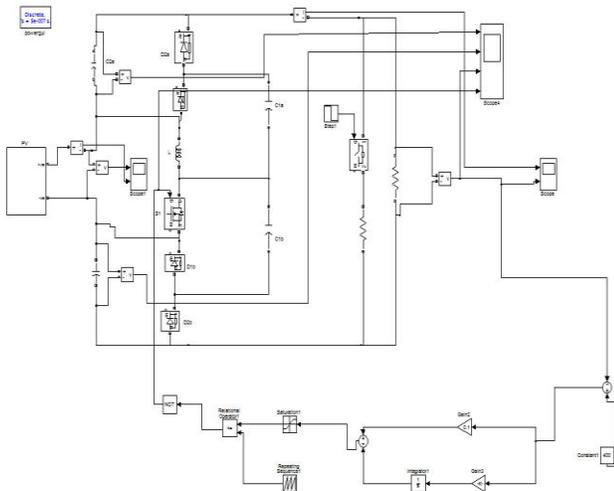
Fig.13 MATLAB/SIMULINK circuit for closed loop control of hybrid boost converttr with PV system
