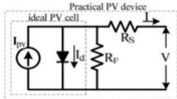
Fig.8 Equivalent circuit of Photovoltaic system.
