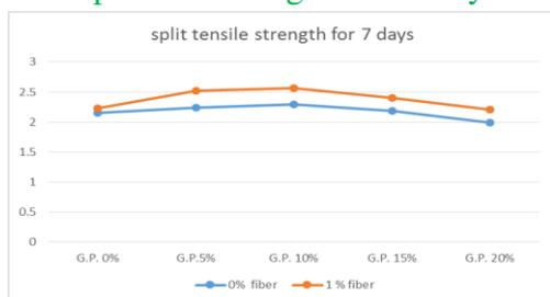
Figure 4.5 Percentage replacement vs tensile strength for 7 days
