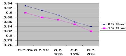
Fig 4.2. Percentage of replacement Vs Compaction factor
