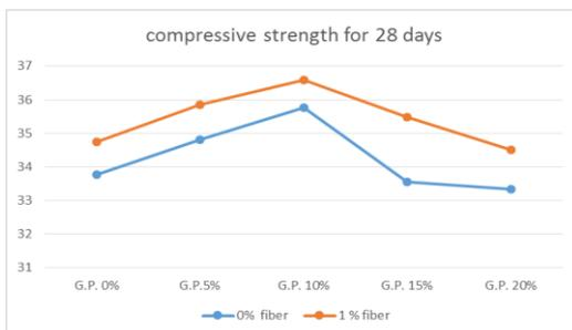
Figure 4.4 Percentage replacement vs Compressive strength for 28 days
