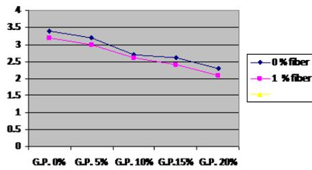
Figure 4.1 % replacement vs slump
