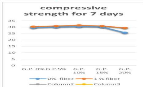
Figure 4.3 Percentage replacement vs Compressive strength for 7 days
