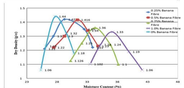
**OMC and MDD values of expansive soil treated with percentage variation of Banana fibre**
