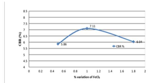
CBR values of Banana fibre treated expansive soil with percentage variation of Ferric chloride.
