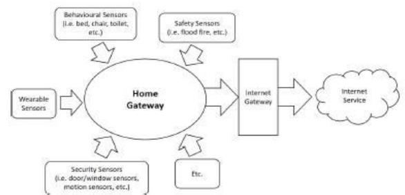
Figure 1: Generic architecture for home sensor network
