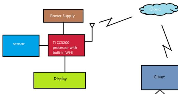
Figure 3: Implemented block diagram Proposed System for active-assisted living
