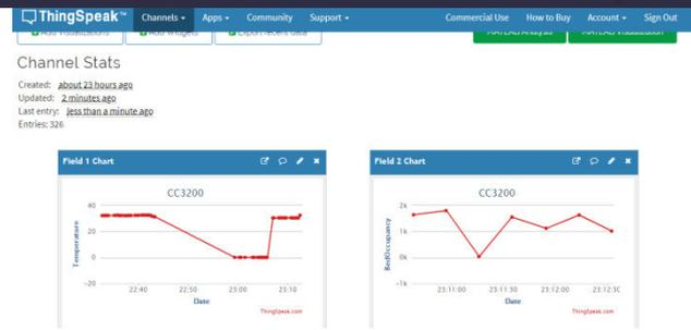
Figure 9: shows the both temperature and bed occupancy data wave forms on ThingSpeak cloud.
