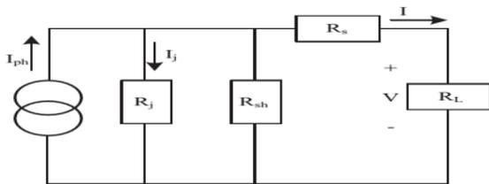
Fig.3 Equivalent circuit of PV array
