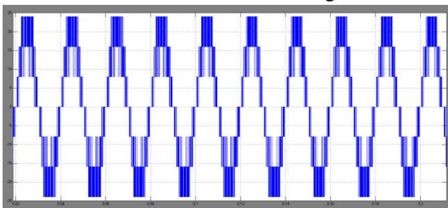
**Fig.16 Output voltage of the seven level inverter**
