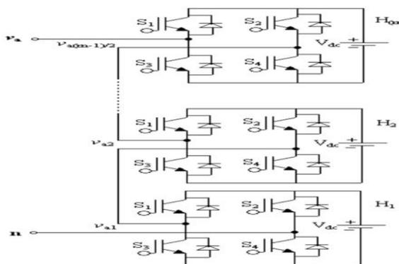
Fig.11 Single -phase cascade multilevel inverter topology.
