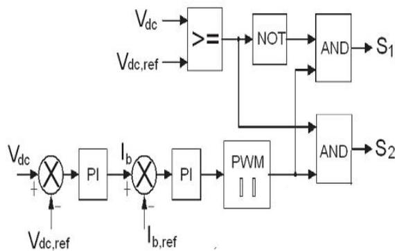
Fig.7. Control of the bidirectional converter
