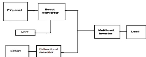
Fig.1. Block diagram of proposed architecture
