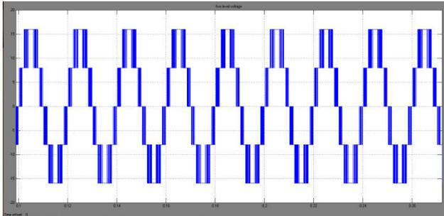
**Fig.14 Output voltage of the five level inverter**
