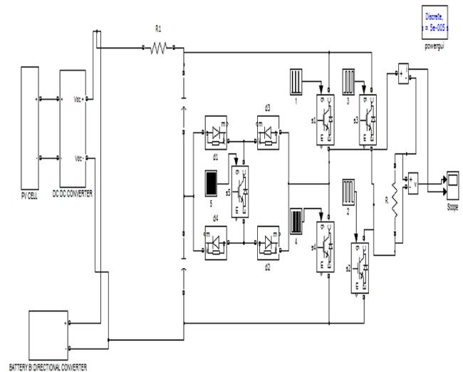
Fig.12 Simulink model of five level inverter
