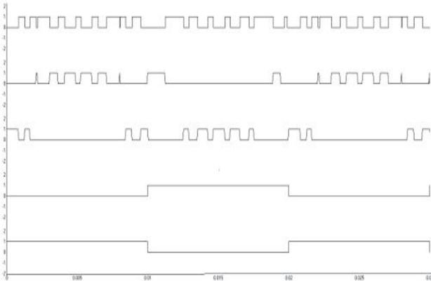
Fig.10. switching patterns of the five level inverter Cascade Multilevel Inverter
