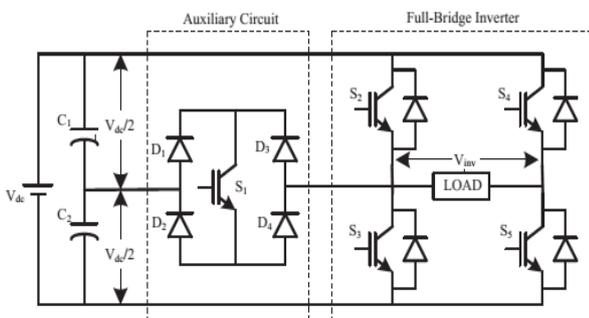
Fig. 8 Circuit diagram of five level inverter
