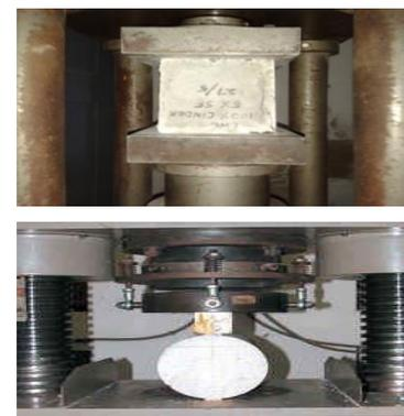
Plate 4.4 Testing of cube Plate 4.5 Testing of cylinder by split tensile
