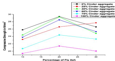
Fig 4.2 Compressive strength with different percentages of cinder aggregate with different percentages of fly ash.
