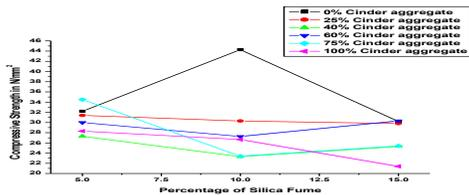
Fig 4.1 Compressive strength with different percentages of cinder aggregate with different percentages of silica fume
