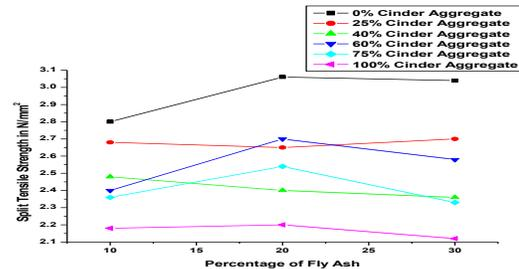
Fig 4.4 Split Tensile strength with different percentages of cinder aggregate with different percentages of fly ash
