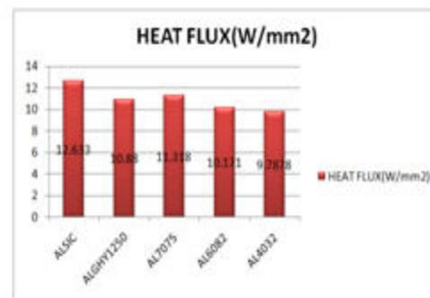
Figure 7 Heat flux
