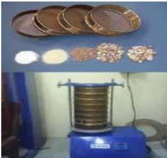
Fig.6. Sieve Analysis of Fine aggregate and Coarse Aggregate
