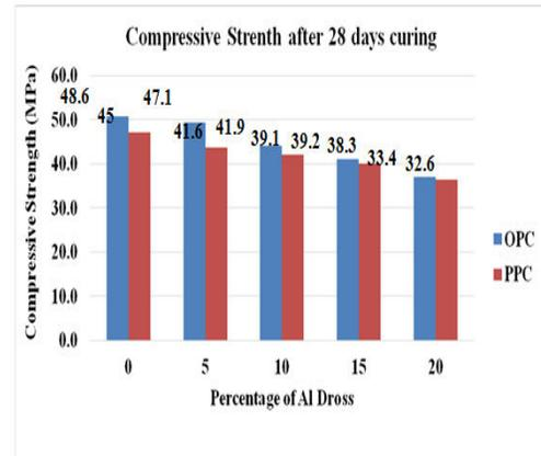
Figure 4. 13 variation of the compressive strength after 28 days of curing for OPC and PPC concrete at various percentage of Al dross
