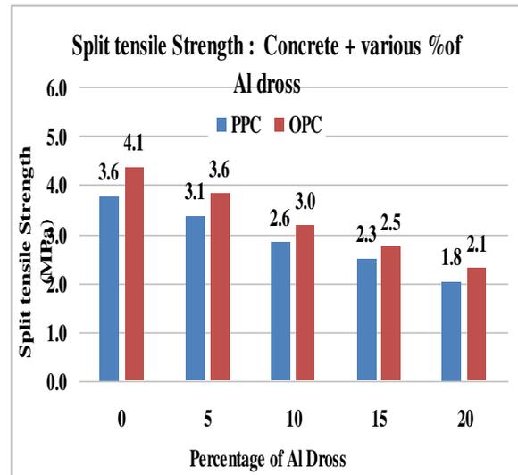
Figure 4. 16 28Days Split Tensile Strength Comparison for PPC and OPC mixes
