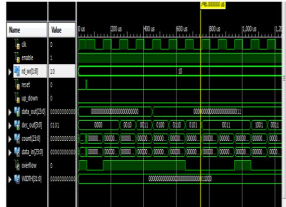
Figure 8 for SRAM read write operation simulation'
