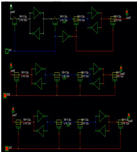
Figure 5 SRAM6T Schematic diagram in back end design
