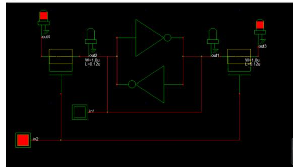
Figure 4 SRAM Schematic diagram in back end design
