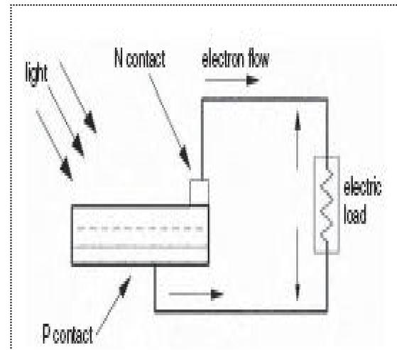
Fig 2.1: PV effect converts the photon energy into voltage across the pn junction
