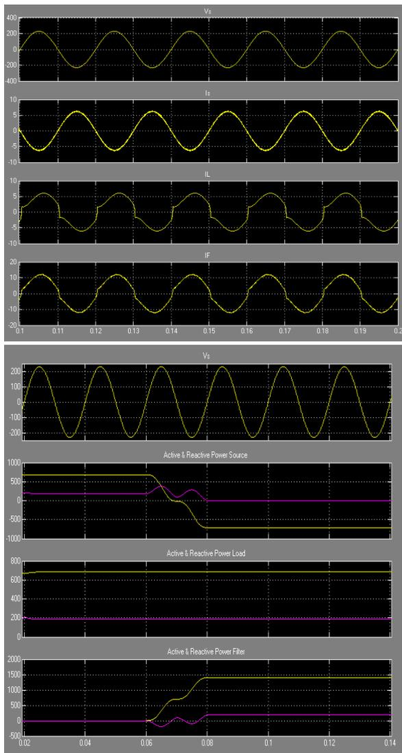
simulation results of the proposed converter under linear load conditions
