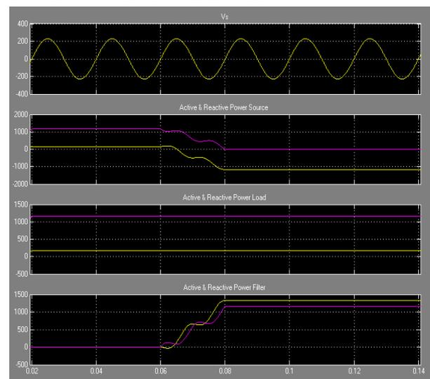
simulation results of the proposed converter under linear load conditions
