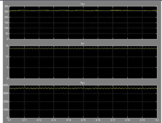
simulated solar PV generating system outputs
