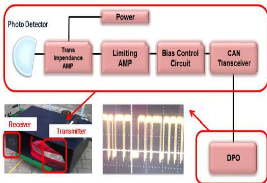
Figure 3. Receiver circuit design and received signal
