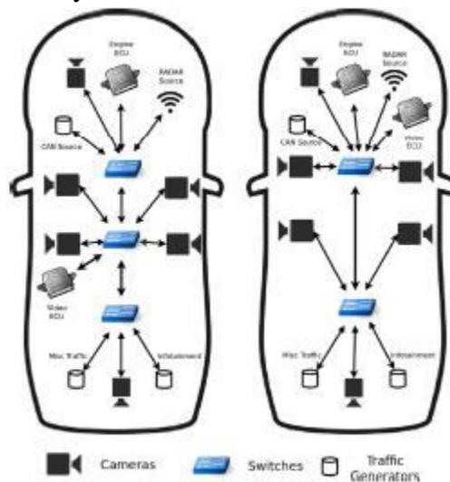
**Fig. 5.** Tested Network Architectures containing cameras, radar, infotainment and CAN sources as well as receiver ECU devices. **Left** - Daisy Chain topology. **Right** - Double Star topology.
