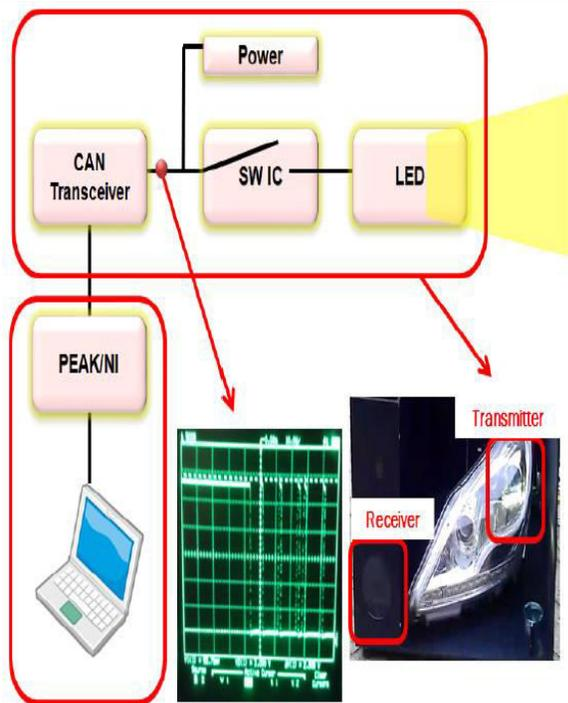
Figure 2. Transmitter circuit design and transmitted signal
