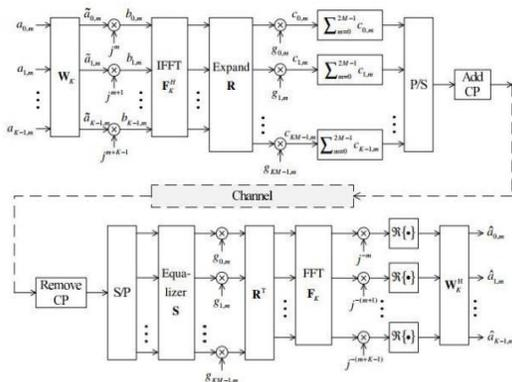
**Fig. 2.1: Equivalent complex baseband WHT-C-FBMC system.**
