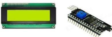
LCDs are useful for creating standalone projects. This LCD Display utilizes an I2C interface, which means that fewer pins are necessary to use this product than would be
