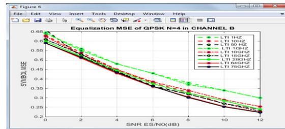
**Fig: 5.8 Equalization MSE of QPSK N=4 in channel B**
