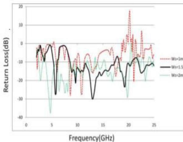
Fig. 2 Simulated return loss(S11) curves for different Ws values
