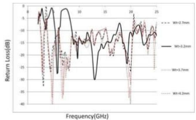
Fig.4 simulated return loss curves for different Wt values
