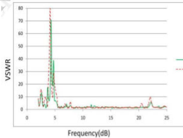
Fig.6. Simulated VSWR for Port1 & Port2
