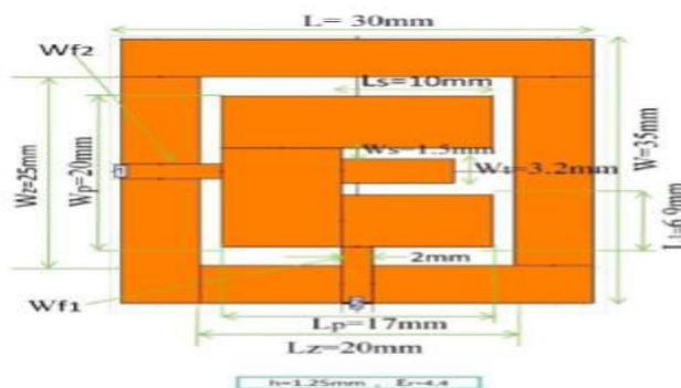
Figure 1. Geometry of the proposed dual feed Microstrip patch antenna
