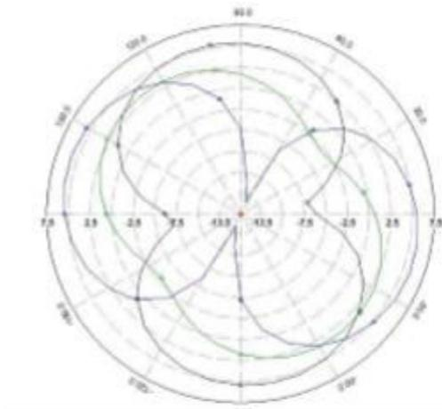
Fig.8. The simulated radiation patterns at different frequencies of .E(x-z) Plane
