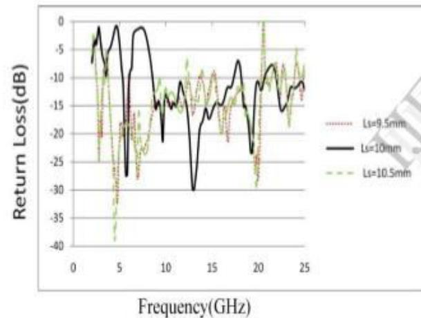
Fig.3 simulated return loss curves for different Ls values
