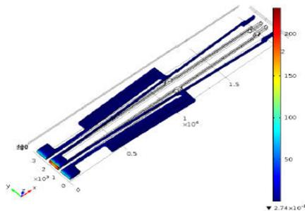
Figure 8: Stress result for 1.2 voltage under simulation
