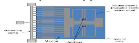
Figure 1. Schematic of comb drive actuator [17]
