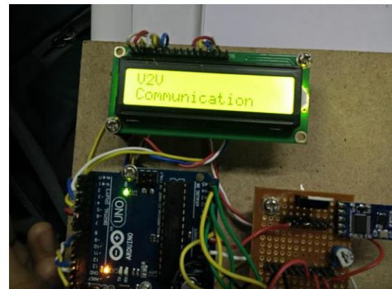
**Fig 4. Message displayed on the on board unit.**
