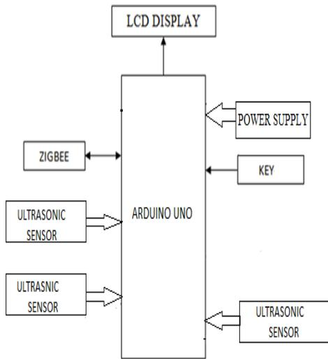
**Fig 3: Block Diagram Of Vehicle On Board Unit (OBU)**
