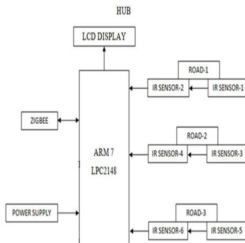
**Fig 2: Block Diagram Of Road Side Unit (RSU)**
