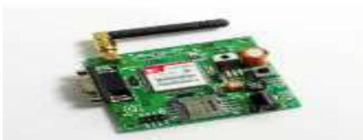
Fig 6.3 GSM Modem
