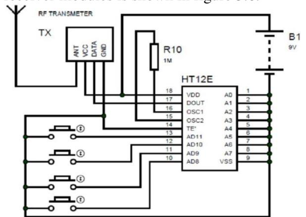
Fig.3.4 RF Transmitter internal schematic
