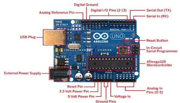
Fig.3.2 Arduino Uno pin description
