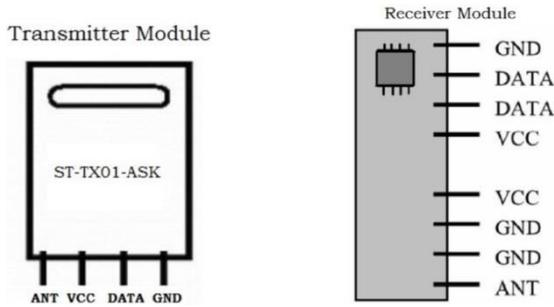
Fig.3.3 RF Transmitter and receiver modules
