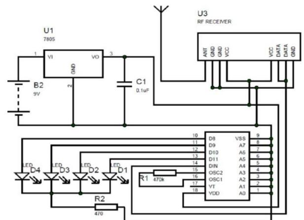
Fig.3.4 RF Receiver internal schematic
