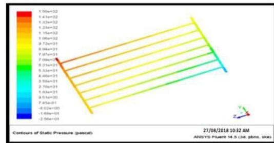
Fig.4.5. Static pressure with fluid water at 90°
