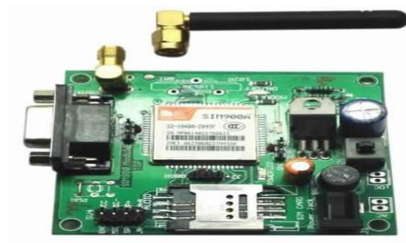
**Fig.7: GSM 900a module**
