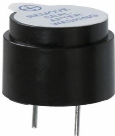
Buzzer is a device which is generally used to produce sound. The operating voltage of is 4-8V DC. The resonant frequency is 2300Hz. The rated current is lesser than 30mA. It is small and neat sealed package. It
