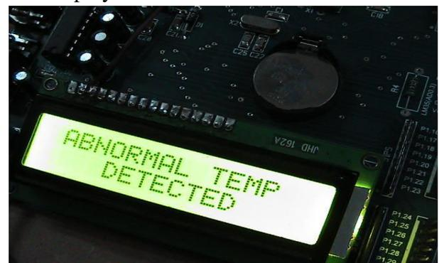
FIG 10 The displayed result when the patient exceeds the standard temperature value:
