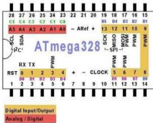
Fig:1: Pinout of ATmega 328
