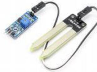
Fig 2: Soil Moisture Sensor
