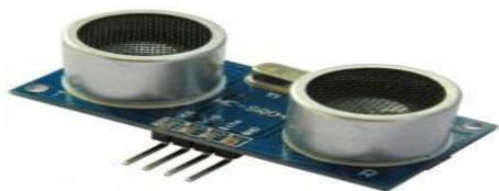
A single I/O pin is used to trigger an ultrasonic burst (well above human hearing) and then "listen" for the echo return pulse. The sensor measures the time required for the echo return, and returns this value to the microcontroller as a variable-width pulse via the same I/O pin.
