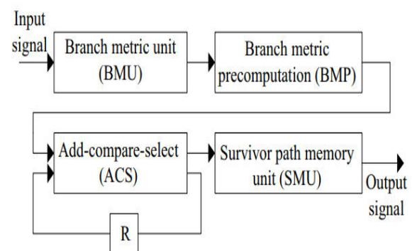
Figure 1.1: Viterbi decoder block diagram. Despite the fact that Viterbi calculation structures are utilized normally in disentangling convolutional codes, within the sight of vast scale joining (VLSI) surrenders, wrong yields can happen which corrupt the exactness in unraveling of convolutional codes.
