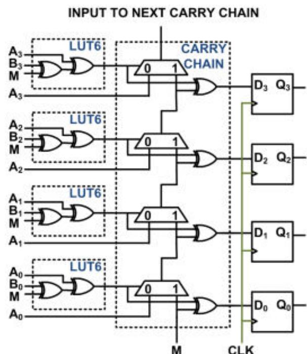
**Fig.3.3. Original pipelined adder subtractor design.**
