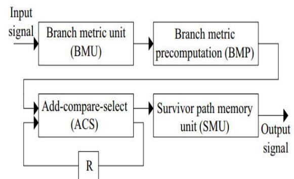
Figure 1.1: Viterbi decoder block diagram. Despite the fact that Viterbi calculation structures are utilized normally in disentangling convolution codes, within the sight of vast scale joining (VLSI) surrenders, wrong yields can happen which corrupt the exactness in unraveling of convolutional codes.
