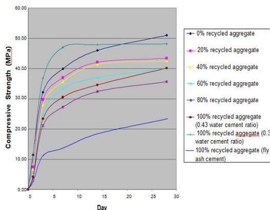
Figure 5.3: Variation of Compressive Strength with
