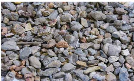
Figure 1.1: Recycled Aggregate.
