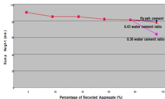
Figure 5.1: Graph showing the result of Slump Test
